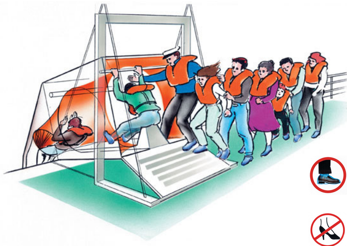
Access through the chute storage box.
