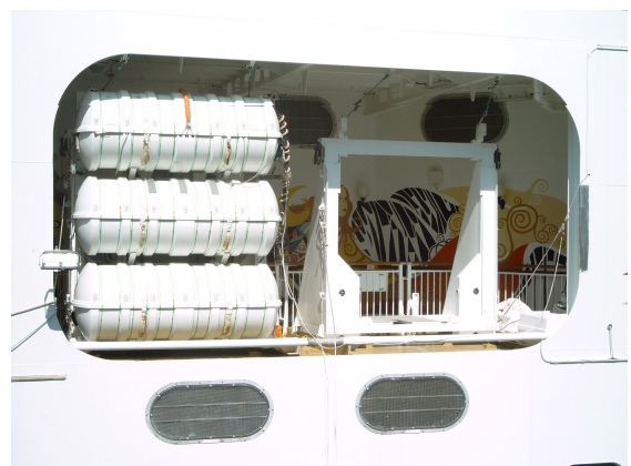
The chute and liferafts can be removed as separate units for servicing. The A-frame remains in position.
