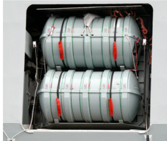
The VEC system can be fitted in an open recess, on open deck or into the ship's side.
